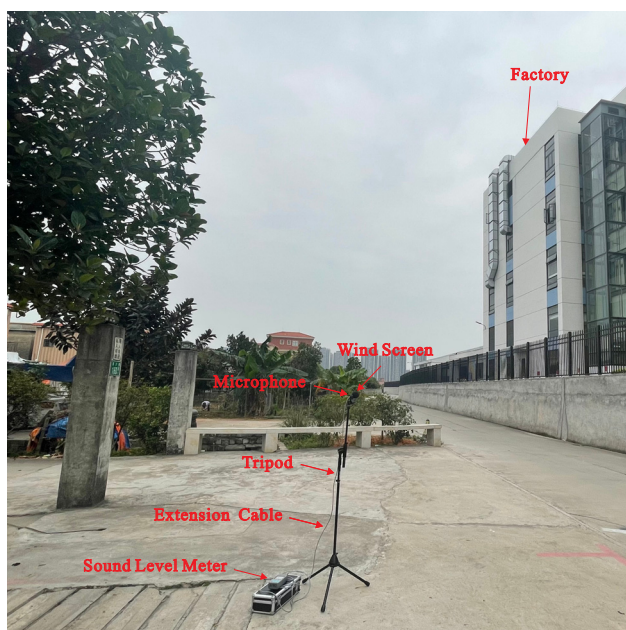
Figure 7: Measurement of the traffic and industrial noise.
