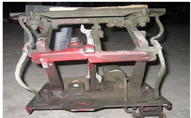
Figure 3: Fracture in the upper frame.
