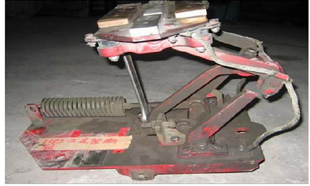
Figure 2: Fracture in the lower frame.
