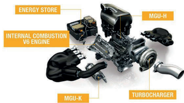
Fig. 1: F1 KERS (ES +MGU-K) and E-BOOST/WHRS (ES+MGU-H) from [8]. The waste energy recovered by the MGU-H and transferred to the ES is minimal and the MGU-H mostly serves as anti-turbo-lag device.
