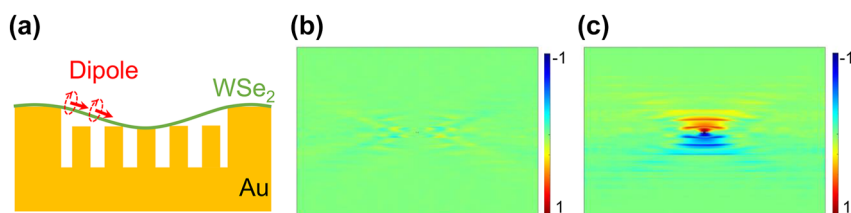
Figure 2: Simulations of electric fields. (a) Schematic of the simulation for a tilted dipole. (b) and (c) Are simulated contrast image of circularly polarized near field ( \rho = (I_R - I_L)/(I_R + I_L) ) under normal and tilted dipole (10°), respectively.
