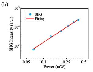
Figure 4: Power dependence of the SHG for LN nanosphere. (a) Measured spectra of SHG under different pump powers at MD resonance. The inset shows the spectral position of the pumping laser with respective of the MD mode. (b) Power dependence of SHG signals in (a), fitted by  $P_{SHG} = mP_{pump}^n$ . The exponent value obtained from the fitting is 2.0.
