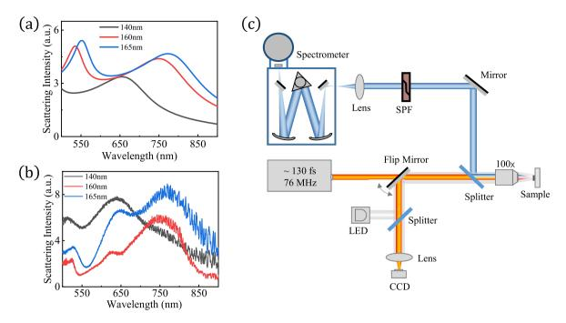
Figure 2: The characterization of the scattering spectra for LN nanosphere. (a) Simulated and (b) experimental scattering spectra of LN nanospheres with different radii. (c) Detection set up for collection of SHG signals from LN nanospheres. The fs incident laser beam is focused on the sample by an objective lens. The reflected incident laser is filtered by a short-pass filter (SPF) and then the backscattered SHG signal is collected by the spectrometer.
