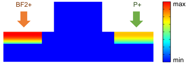
Figure S1. Active dopants concentration (logarithmic scale).
