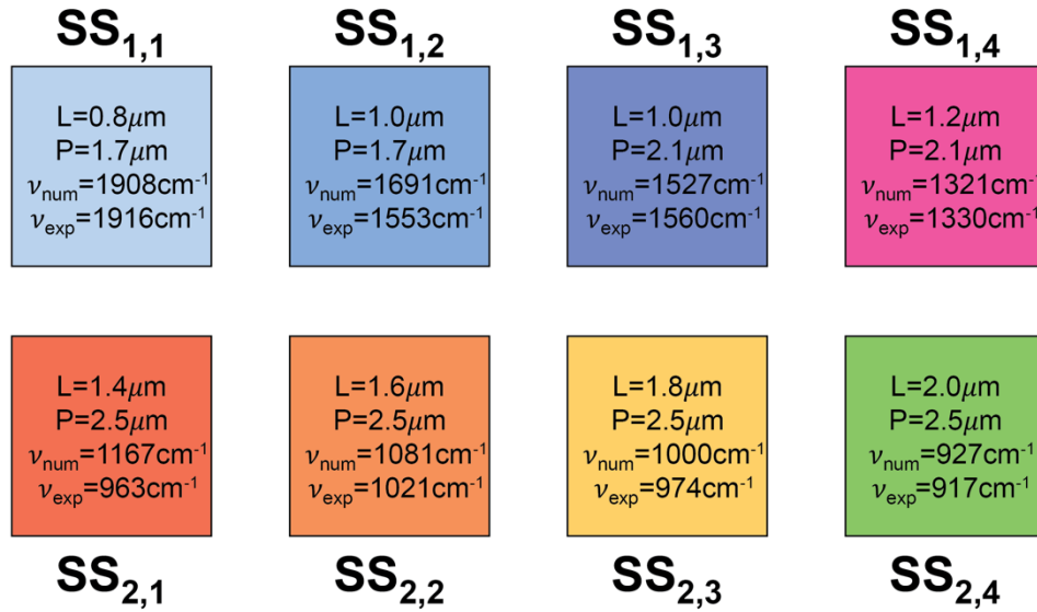
Figure S2: Geometrical parameters pertaining to the SS-type metasurface pixels. The arm width is fixed at W=110 nm. Also shown are the numerical and experimental values of the resonance wavenumber ( \nu_{\text{num}} and \nu_{\text{exp}} , respectively).
