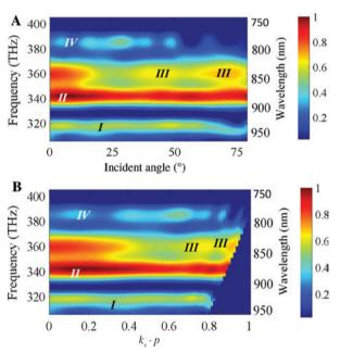
Figure 3: The measured normalized SESHG signal power  $(P_{\rm SH})$  versus the pump frequency (wavelength) and the excitation angle  $\theta$  (A) and equivalent normalized in-plane wavevector (B), showing four important features: (I) a peak in SHG due to the first band edge of the fundamental LP mode, (II) a peak in SHG due to the second band edge of the fundamental LP mode, (III) two peaks in SHG due to PM and (IV) a peak in SHG due to the band edge of the second-harmonic LP mode.
