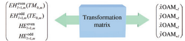
Figure 2: Sketch figure of the transformation matrix connecting l th CV mode bases and OAM mode bases.
