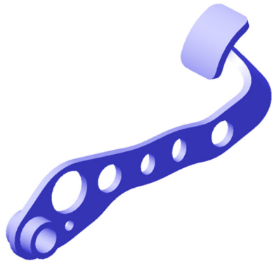
Figure 8: Optimized design of vehicle brake pedal using MHOA.
