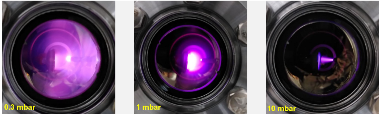
Figure S3: Light phenomena observed under DC gas discharge with N_2 gas at different pressures.
