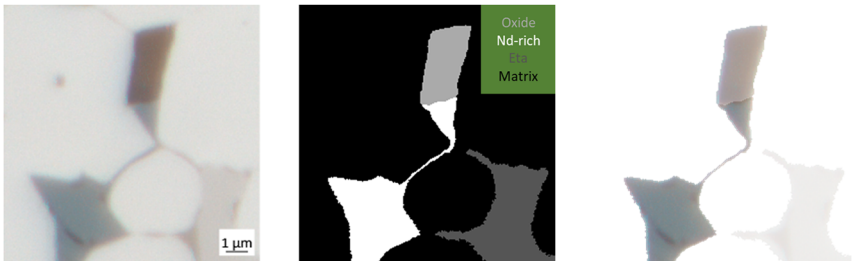
Figure 3: Left: 256 × 256 px RGB patch from the Fe 14 Nd 2 B-magnet image. Center: Mask in grayscale. Color assignments: light gray – oxide, white – Nd-rich, Eta – gray, black – matrix. Right: 4-channel image (combination of the RGB microstructure and mask).
