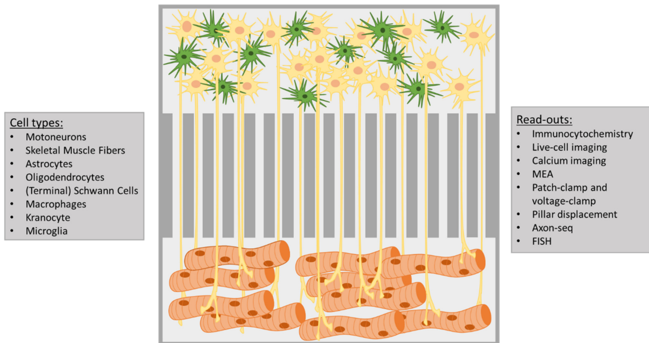
Figure 1: Schematic overview of a simple NMJ-on-a-chip. Motoneurons (yellow) and skeletal muscle cells (brown) are separated by microchannels through which the axons can grow and form neuromuscular junctions. The system can be complemented with additional cell types listed on the left (astrocytes exemplary shown in green). Multiple readouts are possible and dependent on the final design of the platform; possibilities are listed on the right.
