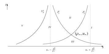
When the projection of  $(\rho_+, u_+, H_+)$  belongs to  $I(\rho_-, u_-) \cup II(\rho_-, u_-) \cup III(\rho_-, u_-) \cup IV(\rho_-, u_-)$  in the  $(\rho, u)$ -plane, the Riemann solution can be briefly expressed by
