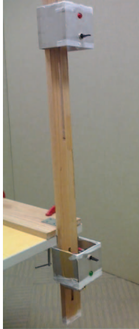
Figure 6. The apparatus used for the non-linguistic contexts ⟨red⟩ and ⟨green⟩, performed by flipping the top and bottom switches on the device, respectively. The distance between the two switches as shown here is approximately 24 inches.
