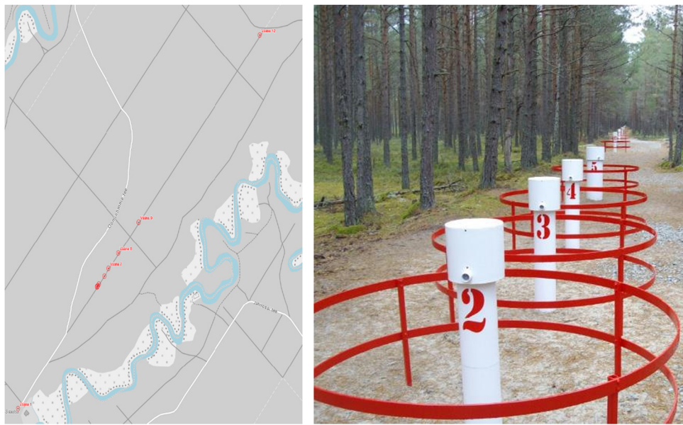
Figure 12: Calibration line in Vääna; on the left, the map view; and on the right, the photo of aligned measurement pillars.
