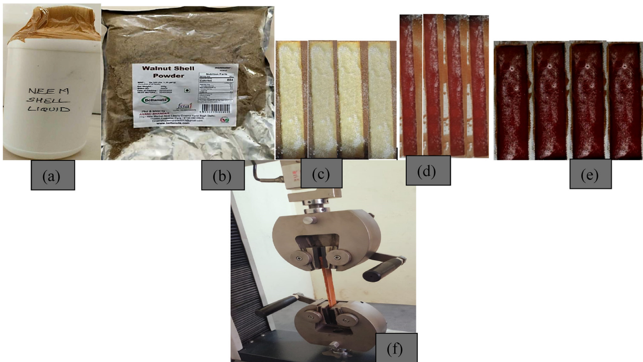
Figure 1: Neem shell and walnut shell powder along with the pure and filler mixed specimens: (a) neem shell liquid, (b) wall nut shell powder, (c) pure neem shell specimens, (d) tensile specimens of neem shell and wall nut powder, (e) flexural specimens of neem shell and wall nut powder, and (f) tensile testing of composite specimen.
