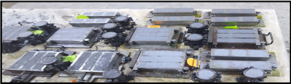
Mixtures after casting in molds according to the dimension of each test
