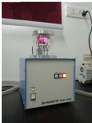
Figure 7: Gold sputter coating process.
