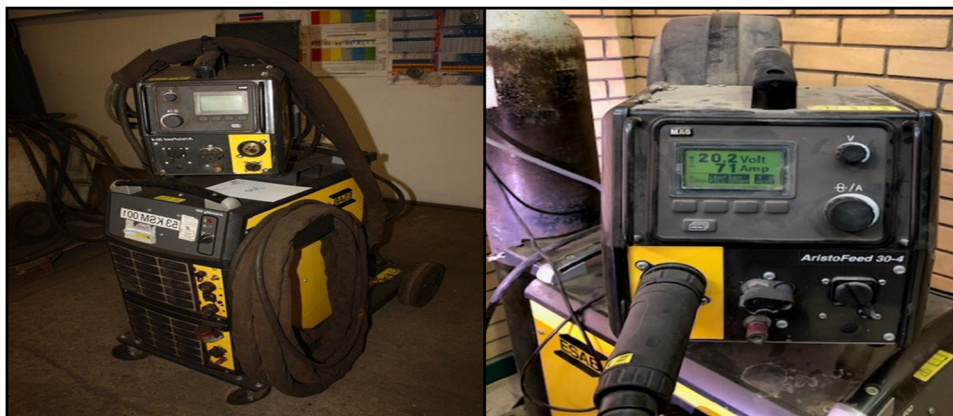
Figure 2: FCAW welding machine used in the experiment.
