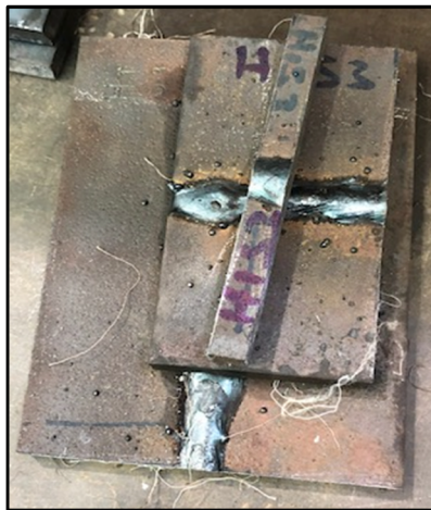
Figure 4: Coupon sampling (transversely).
