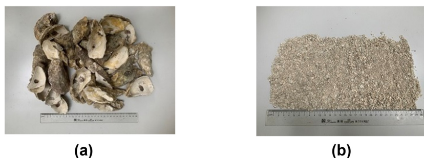
Figure 2: Extraction of Pacific Oyster shell at different scales. (a) Oyster shells are washed and dried before grinding. (b) Grain sizes from 0.15 to 4.75 mm of COSs.
