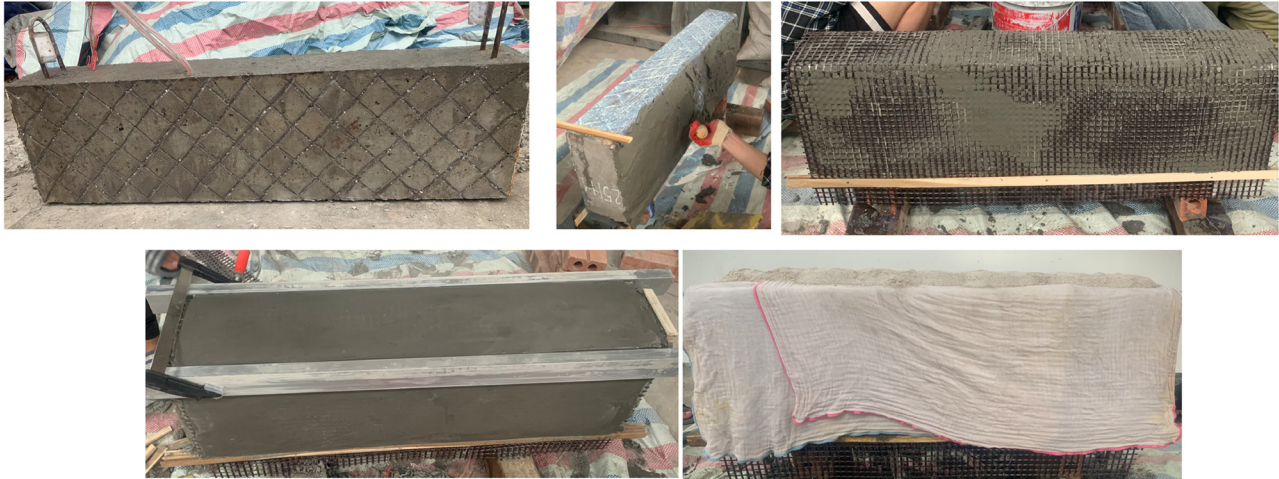
Figure 6: Application of TRC strengthening layers on RC beams.
