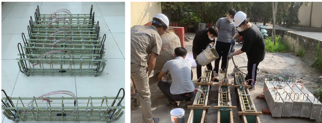
Figure 5: Fabrication of RC beams with COS aggregates.
