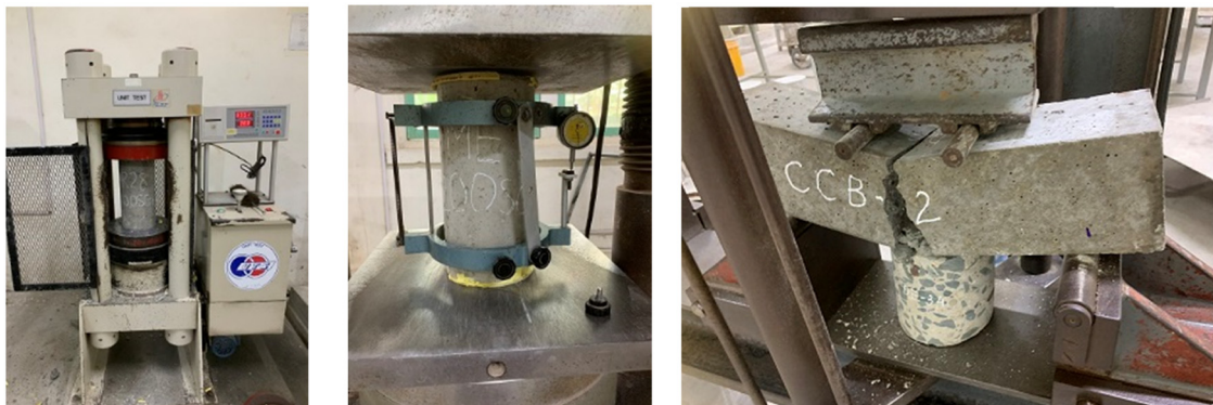
Figure 8: The perspective of experimental work for determining the mechanical properties of traditional concrete and OSC.
