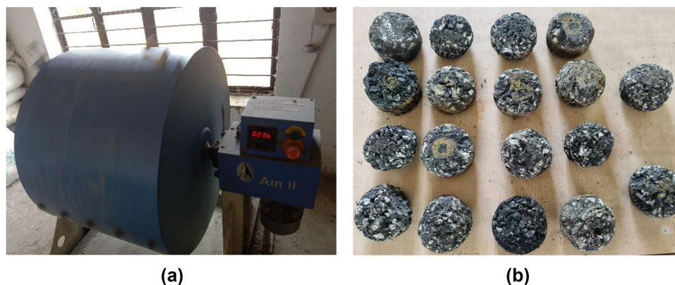
Figure 9: (a) Los Angeles abrasion test machine and (b) samples after testing.
