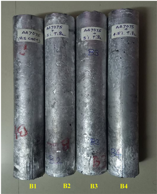
Figure 5: AA7075/TiB 2 squeeze cast composites.
