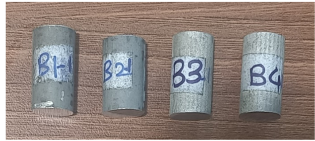
Figure 9: Wear test samples for the AA7075/ \text{TiB}_2 composites.
