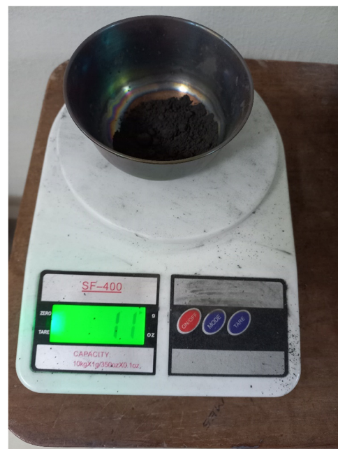
Figure 2: \text{TiB}_2 powder used during the composite manufacturing.
