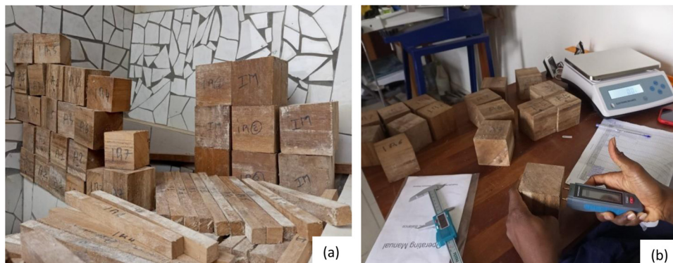
Figure 5: Determination of the physical properties of wood species: (a) cubic wood specimens for the determination of the density and (b) weighing for density and the moisture content evaluation of wood specimens.
