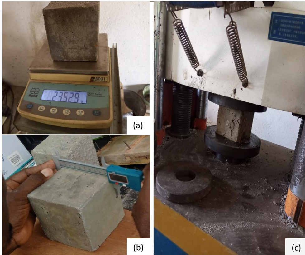
Figure 7: Physical and mechanical characterization of concrete; (a) weight of cubic specimens on a precision scale; (b) reading the dimensions of the test specimens with digital caliper; and (c) compression test on cubic specimens.
