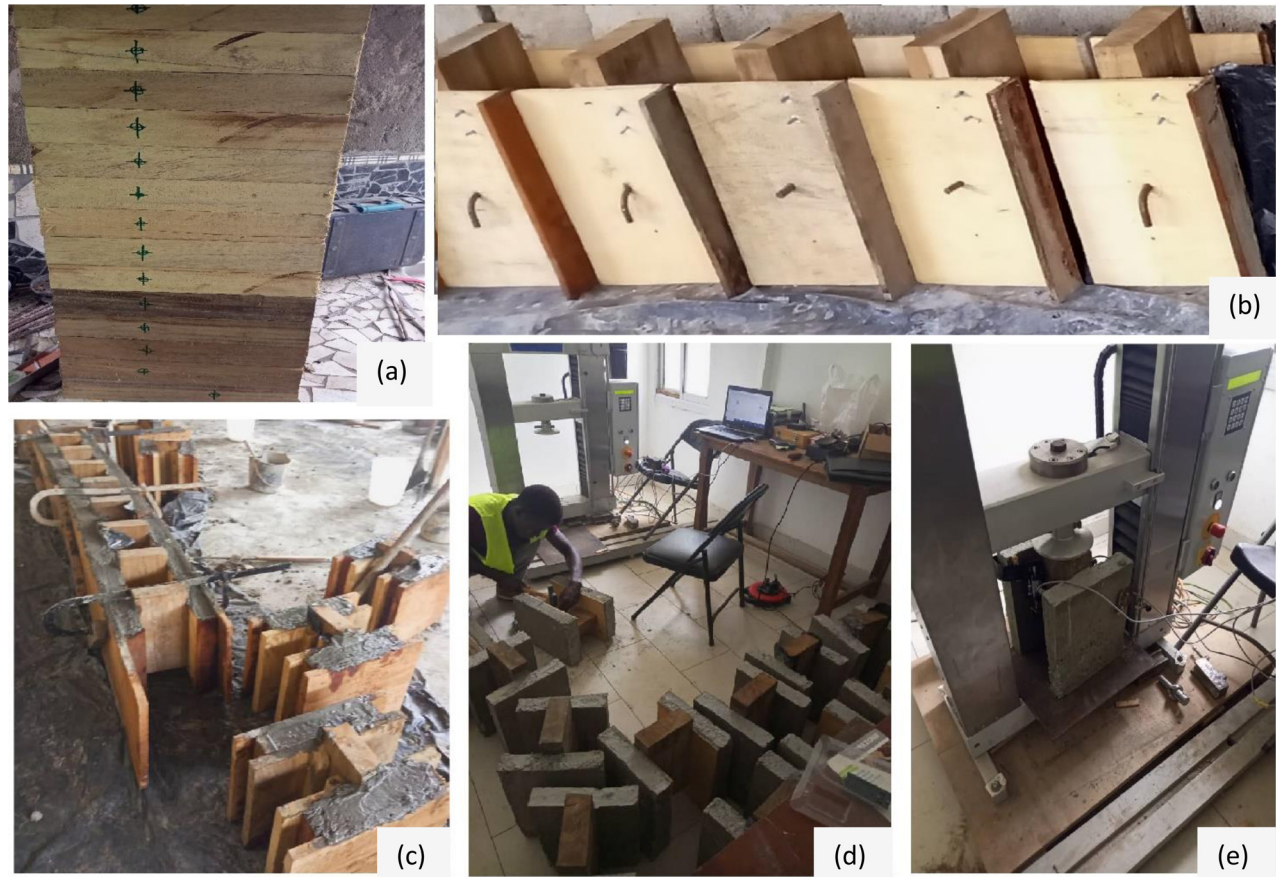
Figure 10: Specimens preparation for double push out tests: (a) marking and pre-drilling of timbers; (b) insertion of connectors in timbers; (c) formwork and concreting of specimens; (d) preparation of the specimens for Push Out tests, installation of potentiometric sensors; and (e) installation of specimens for push out tests on the electromechanical press.
