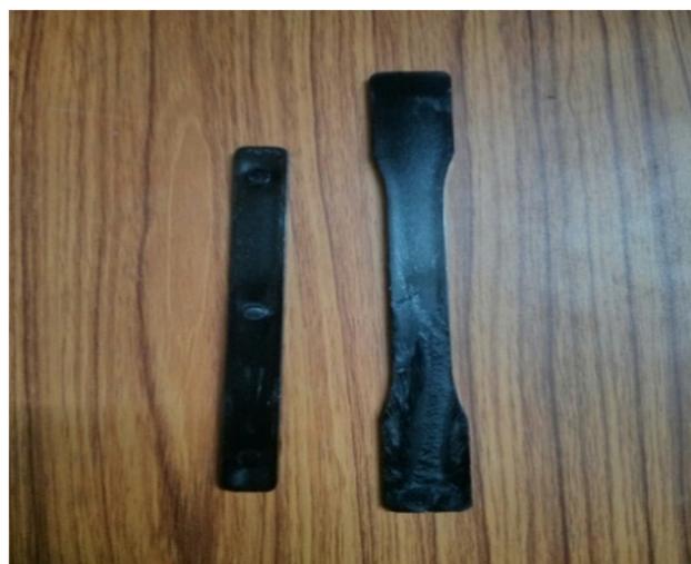
Figure 6: Injection molded test specimens.
