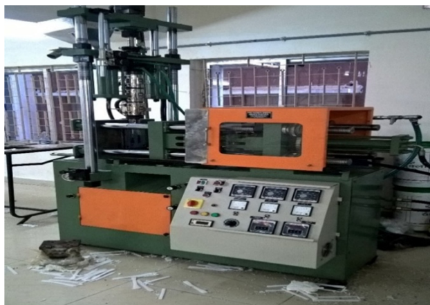
Figure 5: Vertical screw type injection molding machine.
