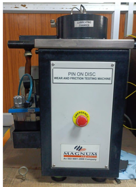
Figure 9: Pin on the disc apparatus.
