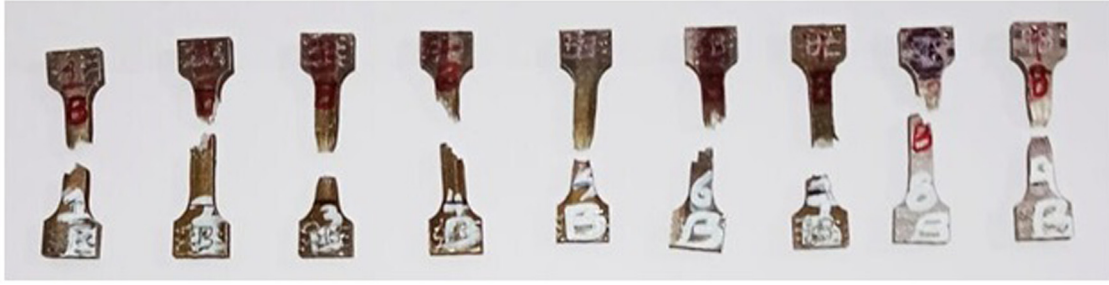
Figure 9: ASTM E8 tensile specimens after failure.
