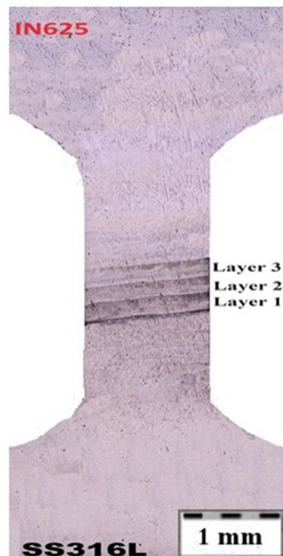
Figure 6: Macrostructure of ASTM E8 sample-6.
