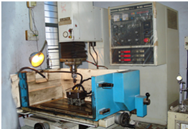
Figure 2: Experimental setup on a Toolcraft V40506 microEDM machine.
