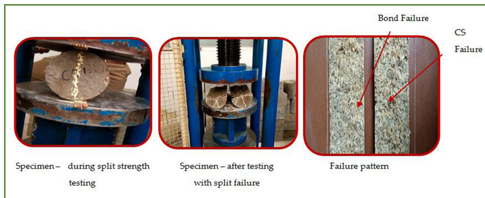
Figure 26: STS – sample specimen – GPCSC mix (M11 – Table 3).
