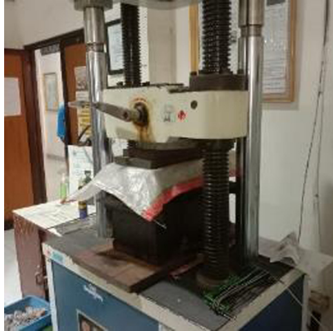
Figure 5: A specimen ready for compressive strength test using micro-computer UTM.
