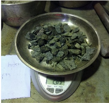
Figure 6: Ballast abrasion test.
