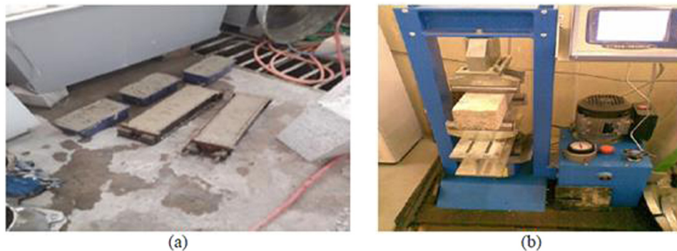
Figure 6: Flexural strength test: (a) prism specimen and (b) flexural testing machine ready to test the prism.
