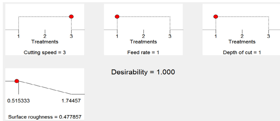
Figure 10: Optimum cutting conditions for surface roughness.
