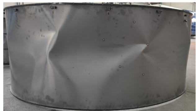
Figure 1: Buckling on pipe [31].
