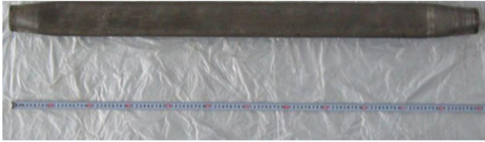
Figure 4: Pipeline failure due to external hydrostatic pressure.
