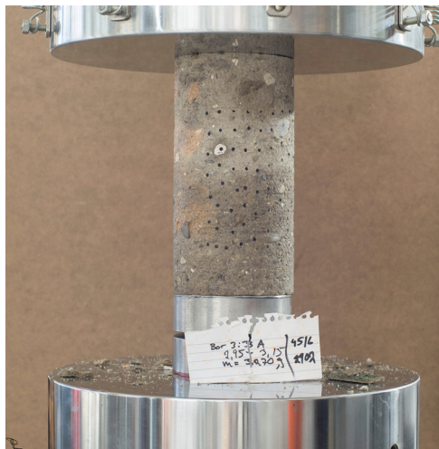
Figure 11: The mechanical press MTS used for UCS test. The axial resonant frequency – 4,516 Hz; flex mode resonant frequency – 2,902 Hz. Photo: Per Lindh.
