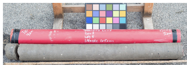
Figure 3: Drill core from the borehole no. 2, depth: between 4 and 5 m. The right part of the drill core consists of natural clay moraine, which is more plastic than the stabilized clay moraine. Photo Per Lindh.
