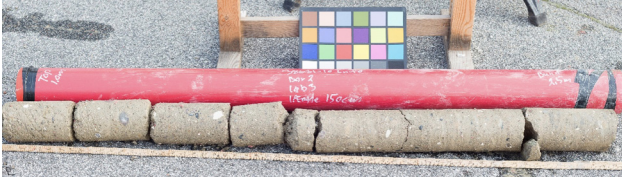
Figure 4: Drill core from the borehole no. 2, depth: between 1 and 2.5 m. The drill core shows homogeneous stabilization along the entire stretch. Photo: Per Lindh.
