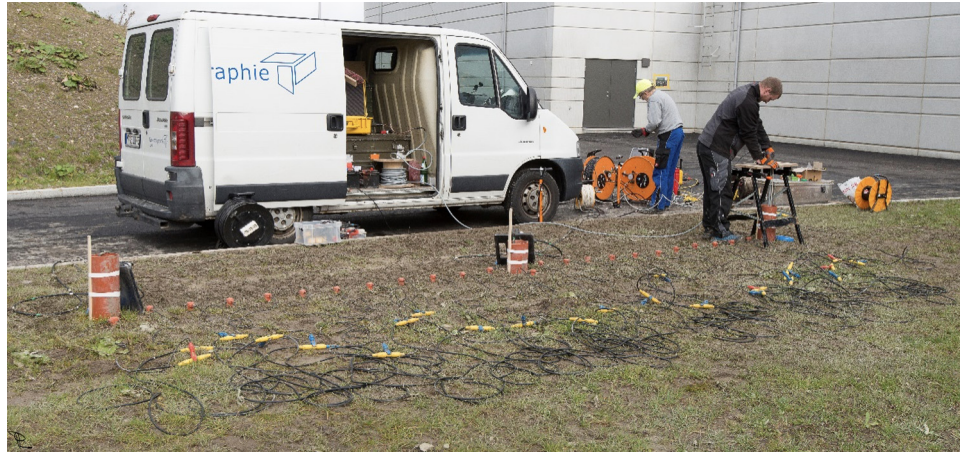
Figure 6: Crosshole measurements on Max IV. The seismic source was located in the borehole No. 1 on the far right of the image. Plastic pipes go down to the stabilized layer. Photo: Per Lindh.
