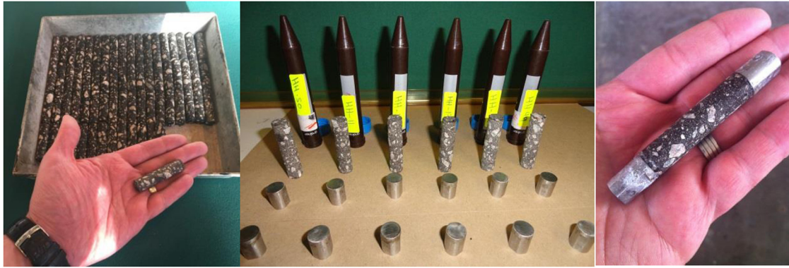
Figure 2: Cylindrical DSR specimens ready for testing.
