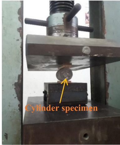
Figure 6: Splitting tensile test.
