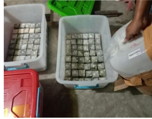
Figure 7: The specimens exposed to NaCl and Na 2 SO 4 solution.
