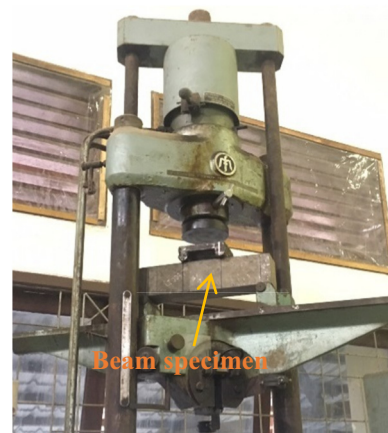
Figure 5: Four-point bending test.
