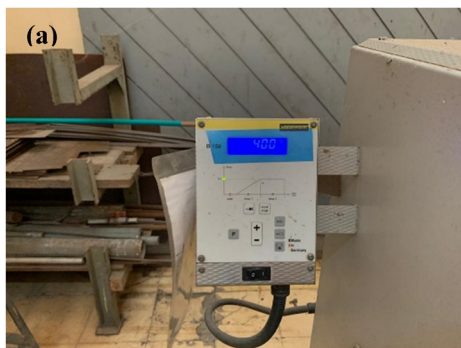
Figure 8: The exposure of the specimens in the laboratory furnace: (a) temperature set up and (b) specimens in the furnace.
