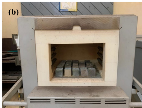
Figure 8: The exposure of the specimens in the laboratory furnace: (a) temperature set up and (b) specimens in the furnace.
