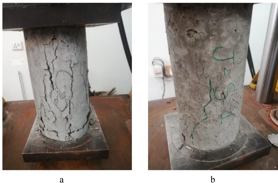
Figure 6: Failure pattern: (a) concrete without coir fiber and (b) concrete with 0.5% coir fiber.
