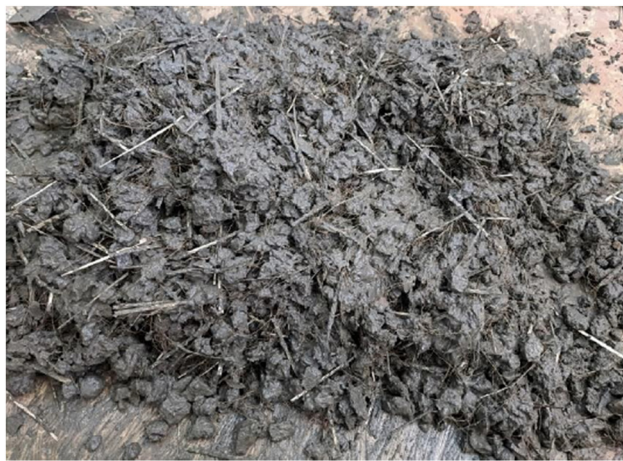
Figure 5: Mixing (coir fiber 0.5% of the total volume of concrete).
