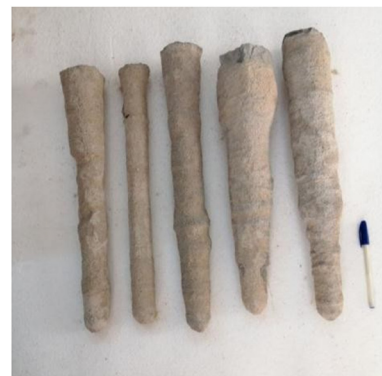
Plate 8: Grouted columns models with diameters of 4–8 cm.
