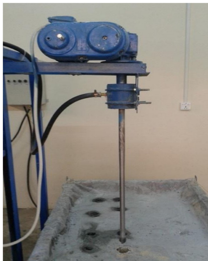
Plate 3: Rotating motor and grouting system.
