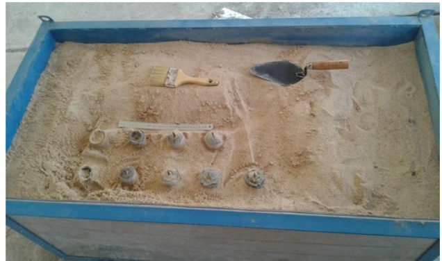
Plate 7: Grouted columns models.
