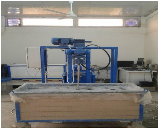
Plate 2: Front view of the low-pressure injection laboratory setup.
