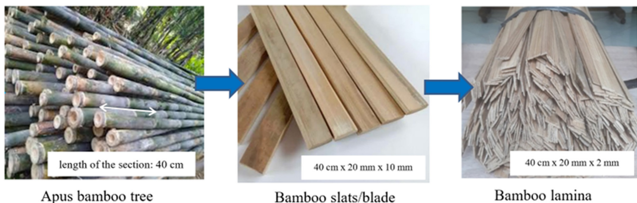
Figure 1: Bamboo lamina-making process.
