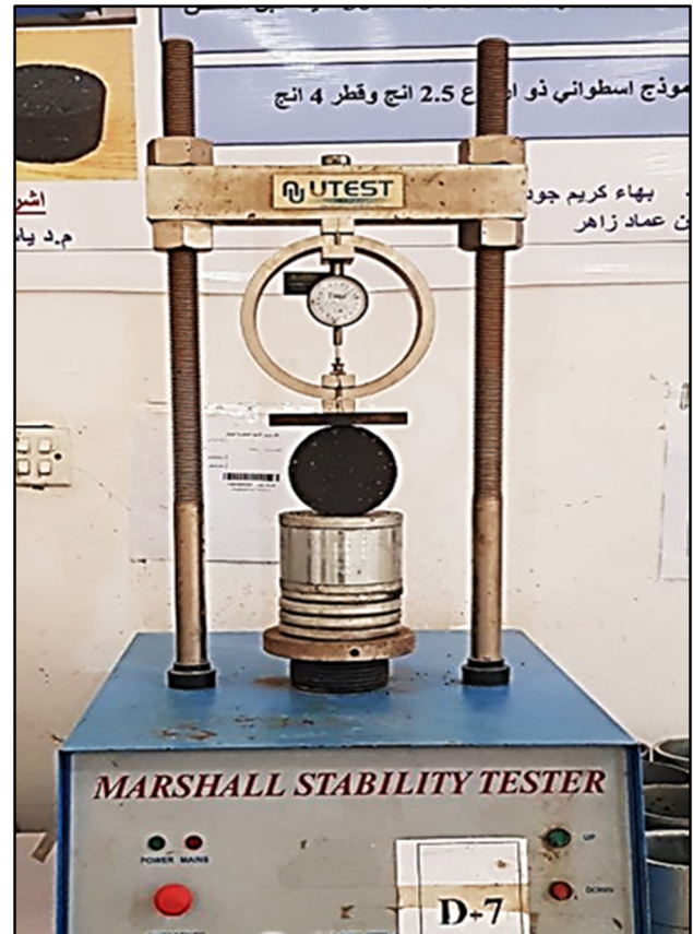
Figure 3: The setup of indirect tensile strength apparatus.
