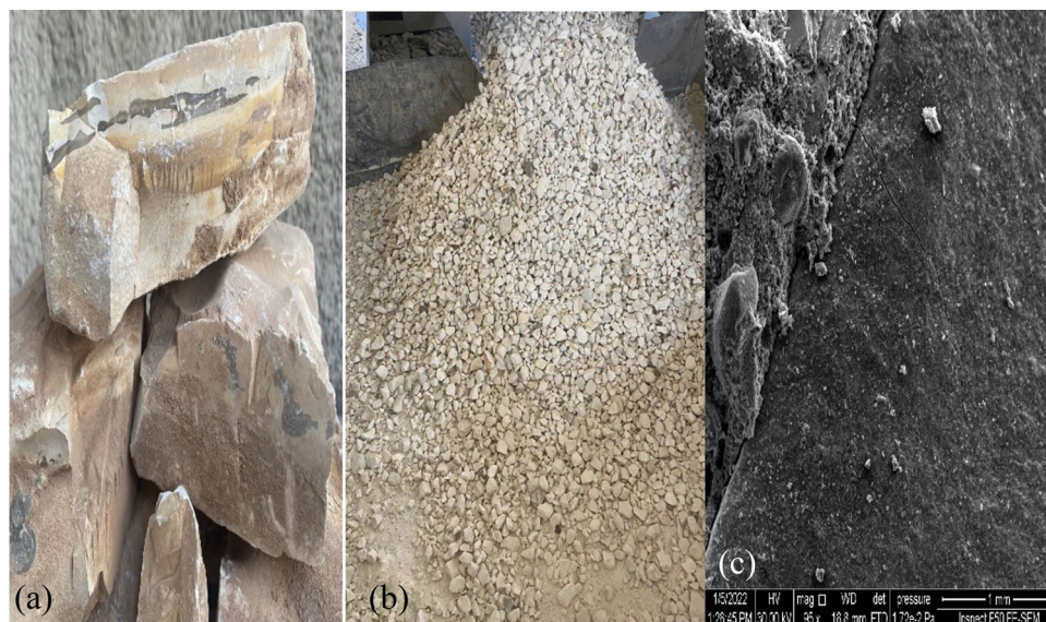
Figure 1: (a) Iraqi porcelanite rock, (b) porcelanite after mechanical crushing, and (c) porcelanite in concrete at FESEM.
