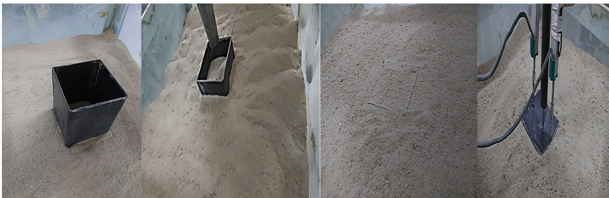
Figure 8: Steps of soil preparation and skirt foundation placement.
