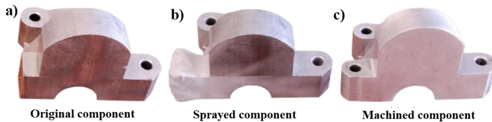
Figure 14: Modification technique of adding a new component to a bearing cap through CSAM [56].
