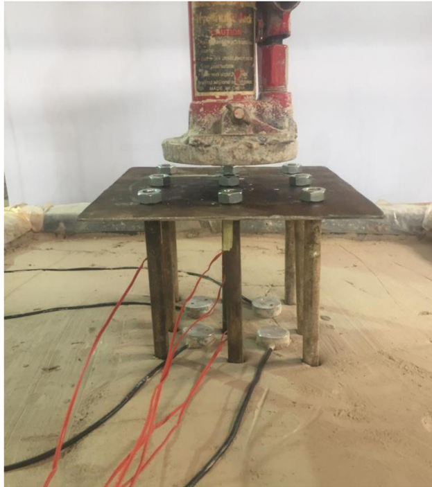
Figure 2: The driving process and instrumentation locations.
