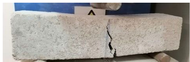
Figure 4: Crack development in a GP-soil beam under flexural loading.
