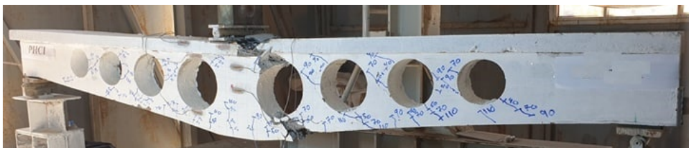
(e) Failure and crack patterns of NPHC8
