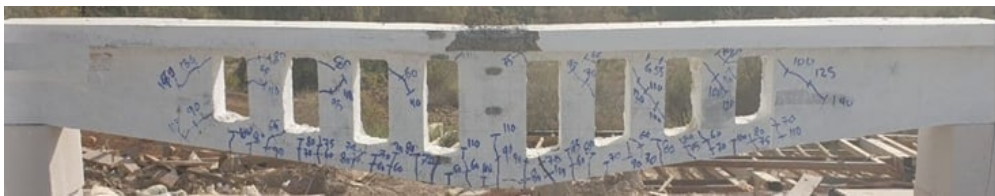
(c) Failure and crack patterns of NPHQ8
