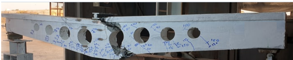
(f) Failure and crack patterns of NPC8
