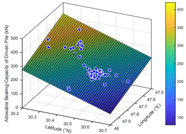
**Figure 9:** Surface defining the variation of the allowable bearing capacity of the driven pile having 9 m length
