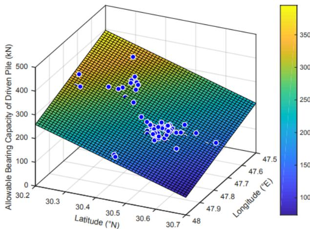
**Figure 8:** Surface defining the variation of the allowable bearing capacity of the driven pile having 8 m length
