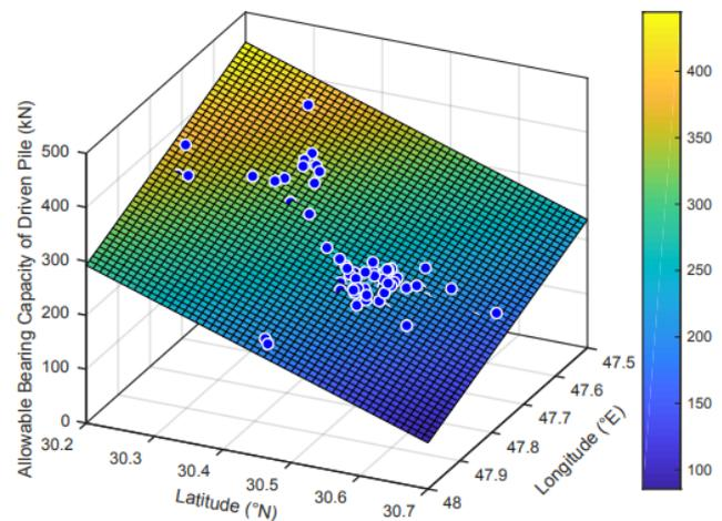
**Figure 10:** Surface defining the variation of the allowable bearing capacity of the driven pile having 10 m length
