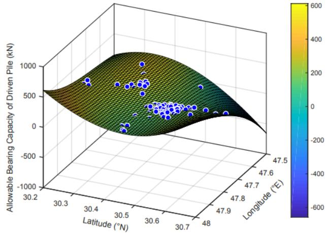
Figure 5: Variation the allowable bearing capacity of driven pile (6 m length) using 3<sup>rd</sup> order polynomial
