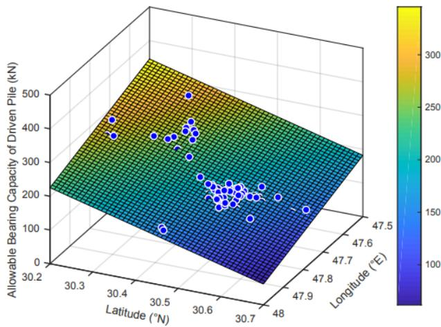
Figure 3: Variation of the allowable bearing capacity of driven piles (6 m length) using 1<sup>st</sup> order polynomial
