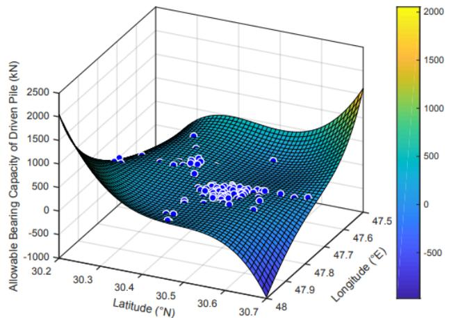
Figure 6: Variation the allowable bearing capacity of driven pile (6 m length) using 4<sup>th</sup> order polynomial
