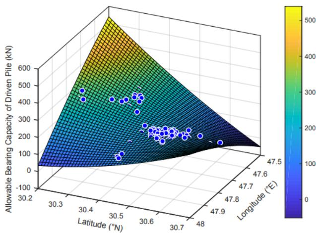
Figure 4: Variation of the allowable bearing capacity of driven piles (6 m length) using 2<sup>nd</sup> order polynomial
