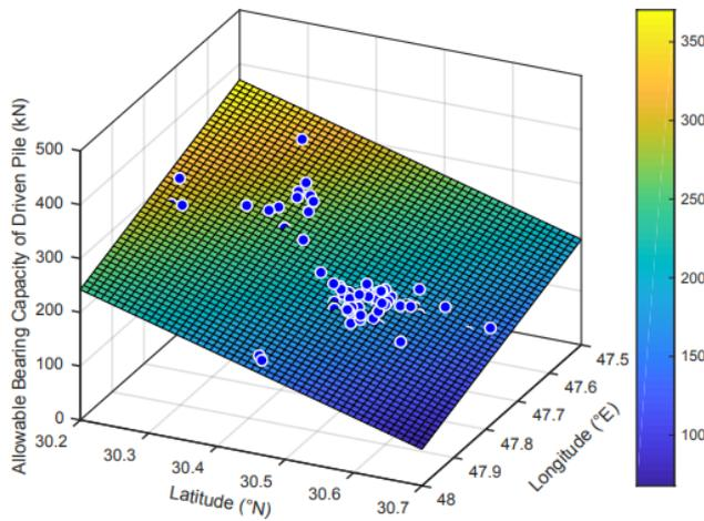
**Figure 7:** Surface defining the variation of the allowable bearing capacity of the driven pile having 7 m length
