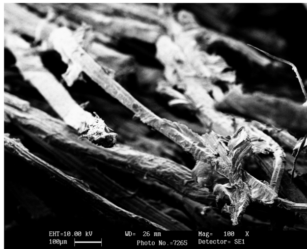
Figure 23: SEM for (5% jute fiber by weight) composite material without coating.
