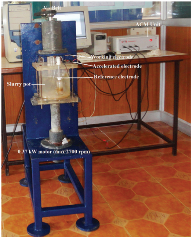
Figure 2: Erosion corrosion test rig.
