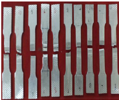
Figure 6: Photograph of fabricated FSW joint (after testing).
